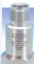
The HS-100I and HS-100SI Series of industrial accelerometers are AC versions which are ATEX and IEC Ex certified for use in Group I and Group II potentially explosive environments. They typically operate over a temperature range of -55 to 140°C and cover a frequency response over 2 Hz to 10 kHz.
